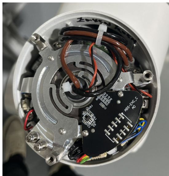
Figure 3-14 : Reconnect the wires
