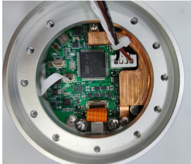
Figure 3-16 : Wires that connect the wrist 3 joints to the end flanges
