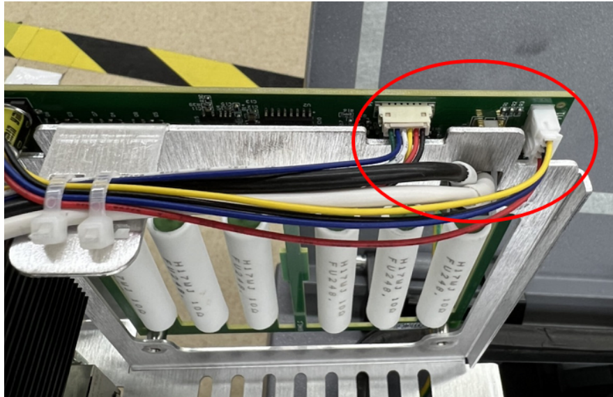
Figure 3-36 : Reconnect the cable
