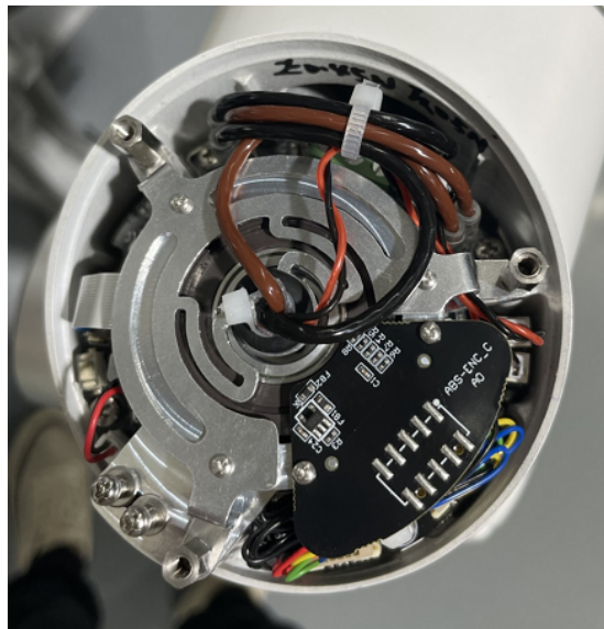
Figure 3-13 : Reconnect the wires
